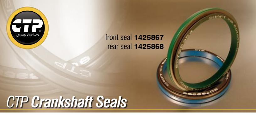
The front and rear crankshaft seals are a proper combination of: Seal + Wear Sleeve. Front and rear crankshaft seals have Wear Sleeves to provide increased crank reusability. Wear Sleeve improves performance of the seal, keeping the dirt away from the sealing lips; this avoids the contamination of oil, maintaining its lubrication properties. The Seal has grooves in the seal lip that return to oil to the deposit during the rotation of the crankshaft.
